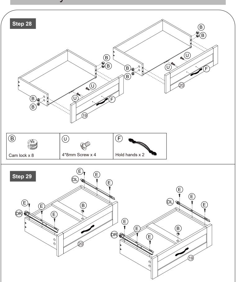
3\*12mm Screw x 12 Runner 300mm x 2 Runner 300mm x 2 Cam lock x 2
